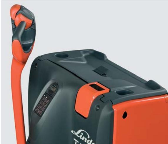
**Storage compartments.** Each truck is equipped with easy-to-reach storage compartments to optimise the operator's work. Wide, deep compartments securely hold items such as shrinkwrap, pens, markers and other equipment.
