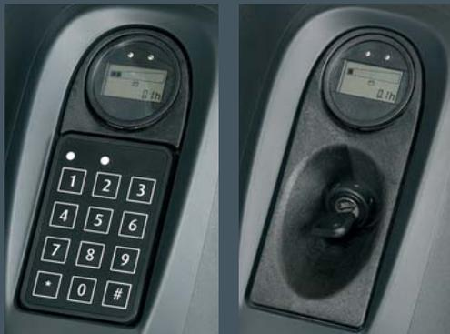
Controlled "Key or Key pad" access. You choose the way to start the truck. Whether by traditional key or by entering a 5 digit PIN-code into LFMgo which is a free of charge option. A large number of access codes can be set to give selected operators truck access but preventing any misuse.
