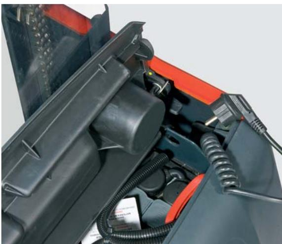
**Built-in charger.** Both trucks can be equipped with built-in chargers for great flexibility allowing charging whenever & wherever needed. The charger cable and socket are neatly stored for easy and safe use. This charger can charge up to 375 Ah both gel and lead batteries at the touch of a switch.
