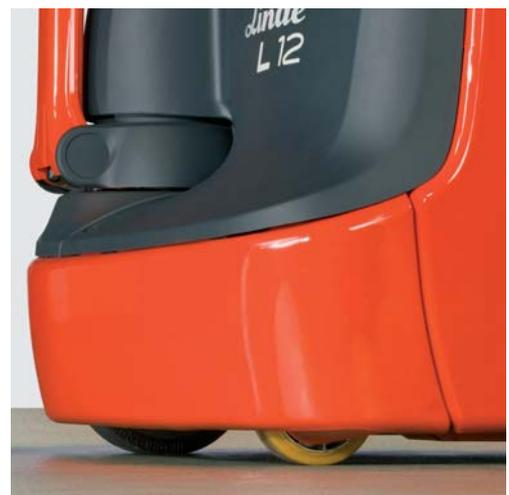
**Safety-oriented construction.** Moulded heavy-duty steel chassis with low skirt, guarantees operator safety by preventing operator's feet becoming trapped under truck.
