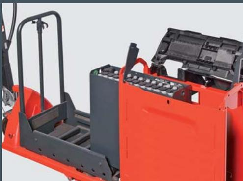
Easy, side battery change. Optional side battery change allows easy battery switching. Easy to operate and safe, the quick change feature allows the battery to be rolled off to either side of the truck. Its special locking system ensures that the battery is securely kept in place. As standard, vertical battery change is also available.
