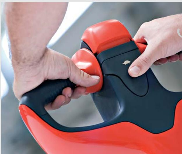
**Creep speed.** The Linde Creep speed feature allows the truck to manoeuvre in confined areas with the tiller in an upright position, normally one of the braking zones. By activating the Creep speed button, easily accessible by either hand, a top speed of 1.5 km/h is set for the truck. The operator can then freely operate and easily manoeuvre the truck on a tail-lift while loading or unloading.
