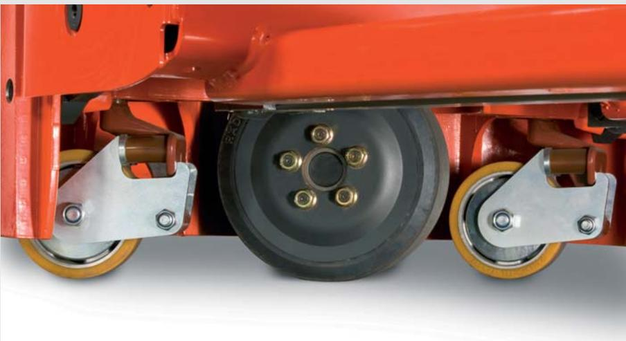
**Castor wheels.** Three-wheel configuration with two adjustable castor wheels leads to perfect traction behaviour. The castor wheels are larger and mounted on shock absorbers to maintain truck stability while handling loads.
