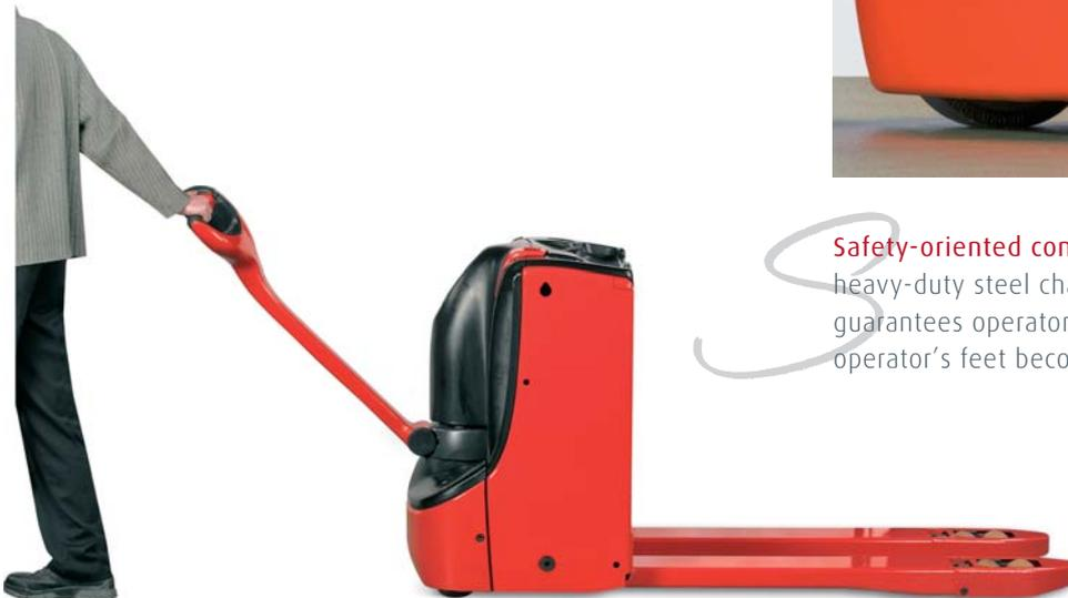
**Long tiller & low mounting.** A long tiller arm with a low mounting point ensures a large safety clearance between operator and chassis, as well as providing light steering for sharp corners.
