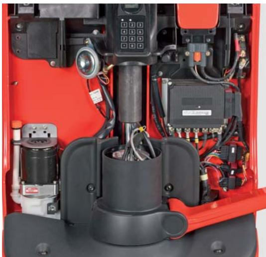
**Quick access, reduced wear.** The motor service panel provides fast and easy access to all internal components. As all electrical cables are sheathed, service work can be handled fast. The electromagnetic braking system extends maintenance intervals by reducing wear and tear.
