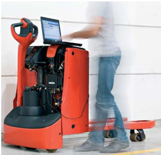
**CAN-bus architecture.** Besides quick adjustments to operating parameters, intelligent CAN-bus technology also provides a broad spectrum of state-of-the-art truck diagnosis and maintenance functionality. It carefully monitors all key functions for quick and simple diagnosis by a service engineer.
